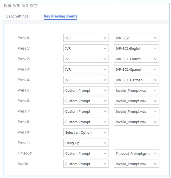
Figure 14: IVR-SC2 Key Pressing Events Configuration
