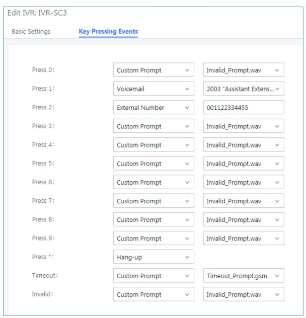
Figure 17: IVR-SC3 Key Pressing Events Configuration
