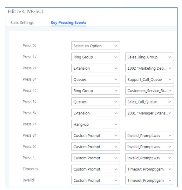
Figure 10: IVR-SC1 Key Pressing Events Configuration
