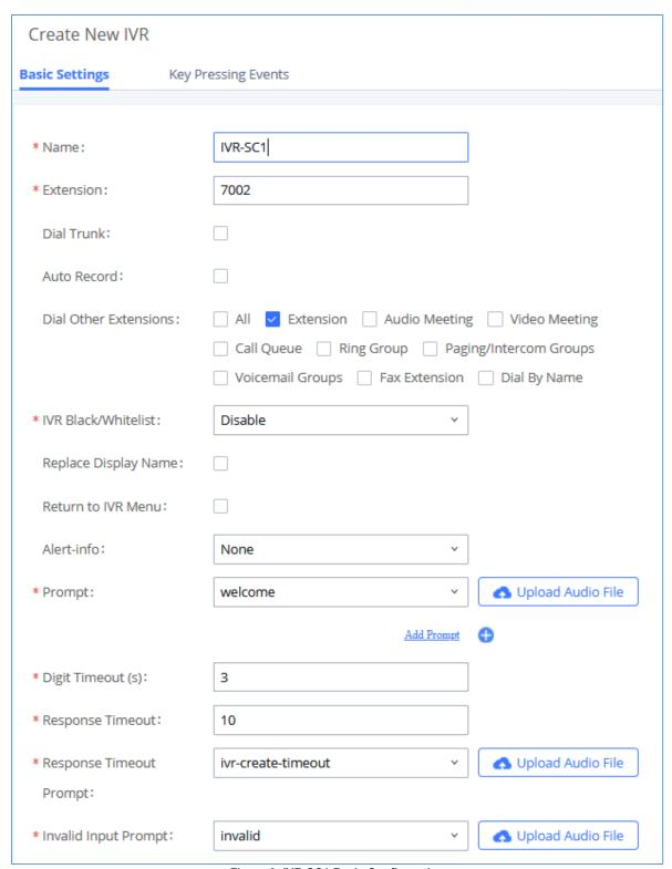
Figure 9: IVR-SC1 Basic Configuration
