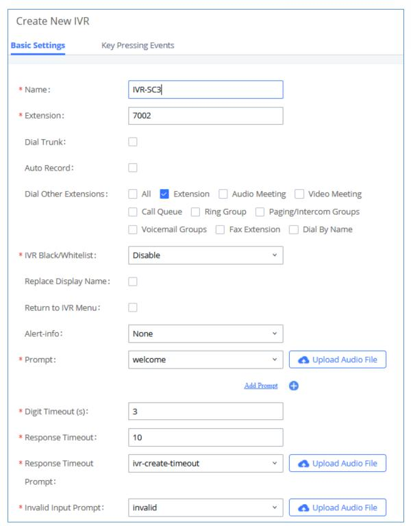
Figure 16: IVR-SC3 Basic Configuration
