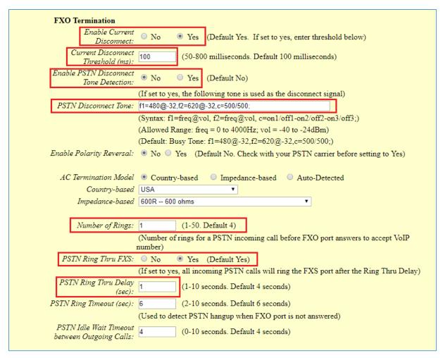
Figure 8: Configure FXO Port on the HT813 - FXO Termination
