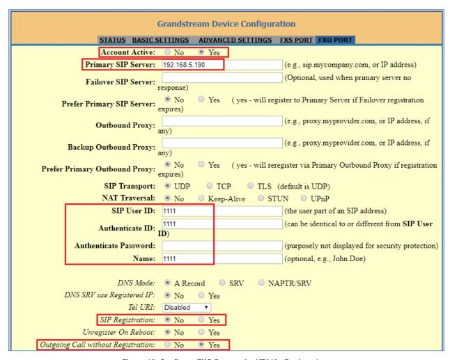
Figure 15: Configure FXO Port on the HT813 - Registration
