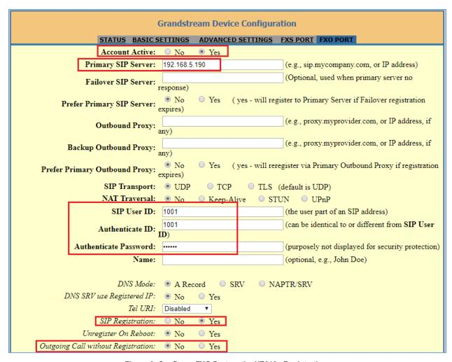
Figure 6: Configure FXO Port on the HT813 - Registration
