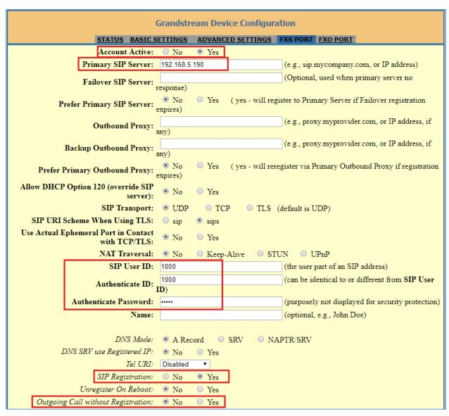
Figure 5: Configure FXS Port on the HT813
