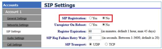
Figure 6: Configure FXO Port on the GXW410X - SIP Settings
