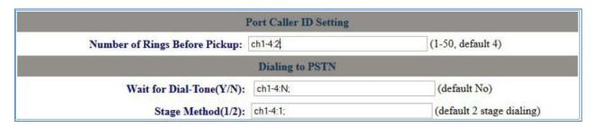
Figure 11: Configure FXO Port on the GXW410X - FXO Termination
