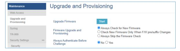
Figure 2: Option "Firmware Upgrade and Provisioning" - GRP261x, GRP2624 and GRP2634
