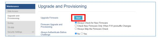
Figure 26: Manual Upgrade Start Button on GRP261x, GRP2624 and GRP2634
