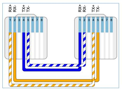
Figure 3: T1 Crossover Cable Pin-out
