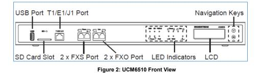
Use a T1 crossover cable to plug one end into the UCM6510 T1/E1/J1 port. Plug the other end into the T1/E1/J1 walljack. Please check if the T1 crossover cable can be provided from the service provider. The proper T1 crossover cable pin-out is shown in the following figure.
