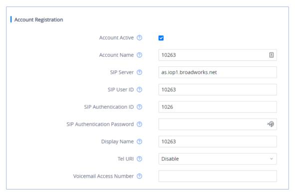
Figure 6: Configure SIP Account Setting for Secondary Phone
