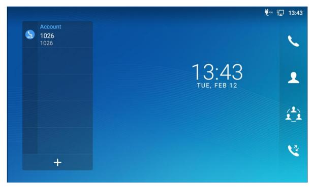
Figure 5: Account Icon in the Widget When Turn on SCA Feature
