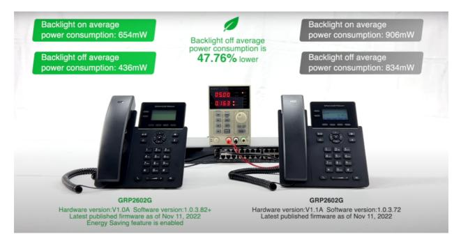
Alternatively, the illustration below compares the power consumption of grandstream carrier-grade and other competitors' IP phones.
