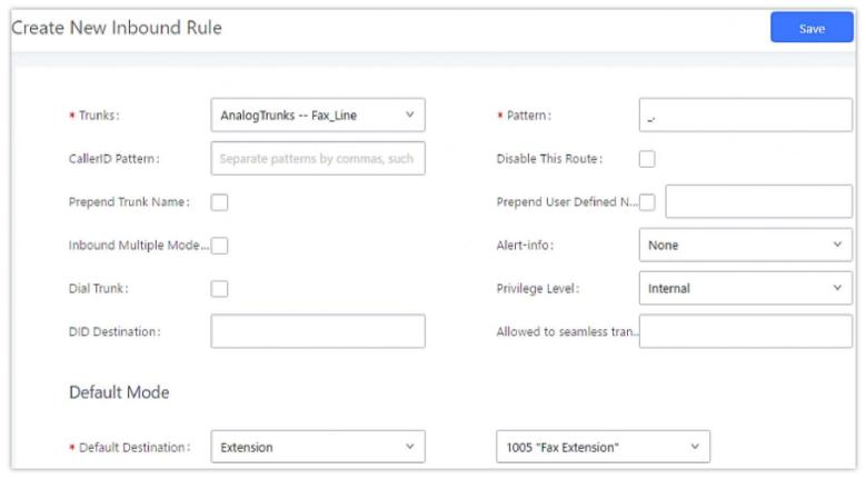
Figure 212: Configure Inbound Rule for Fax
