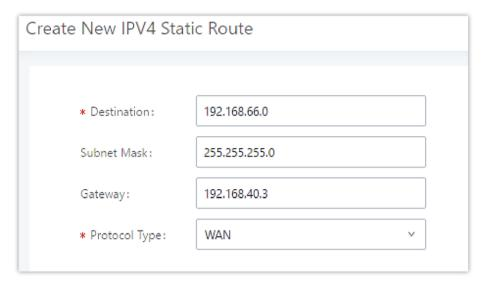
Figure 18: UCM6510 Static Route Configuration
