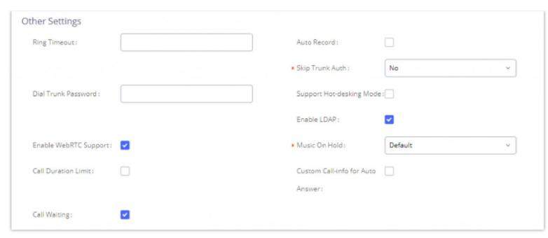
Figure 155: Enabling WebRTC on extensions
