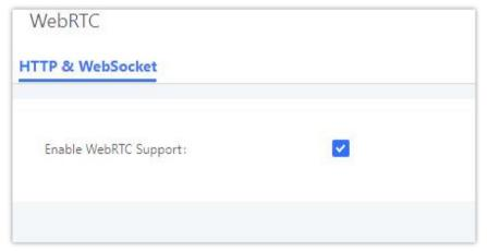
Figure 154: Enabling WebRTC feature
