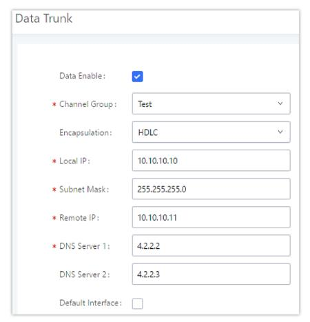
Figure 108: Data Trunk Configuration
