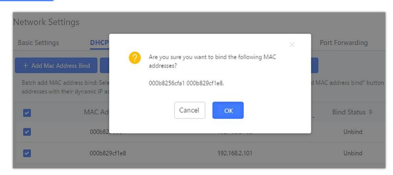
Figure 14: Batch Add MAC Address Bind
