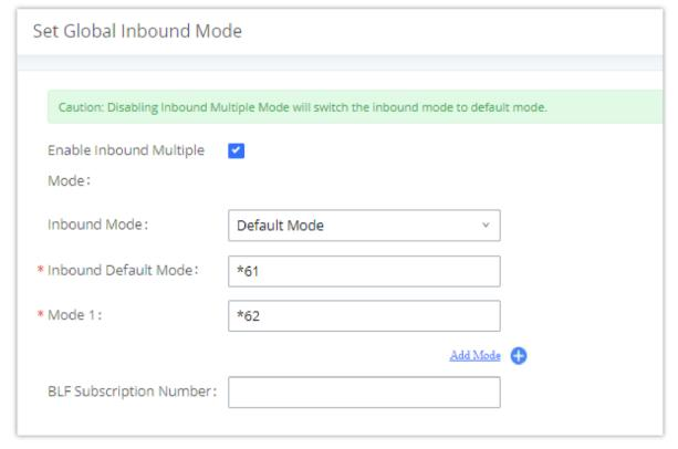
Figure 132: Inbound Route - Multiple Mode Feature Codes
