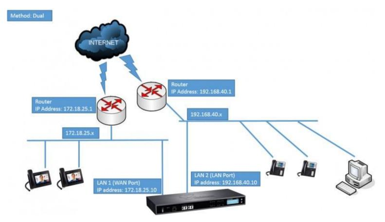
Figure 11: UCM6510 Network Interface Method: Dual
