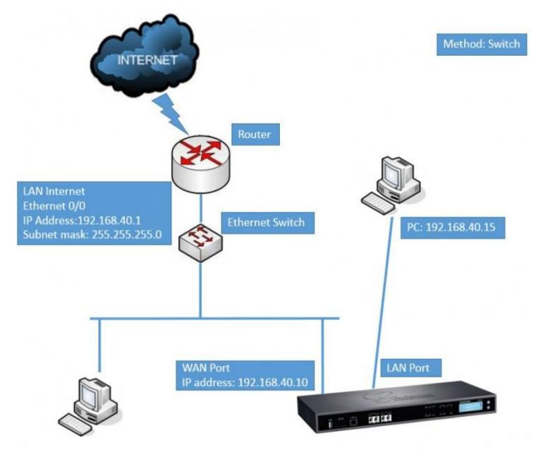
Figure 10: UCM6510 Network Interface Method: Switch
