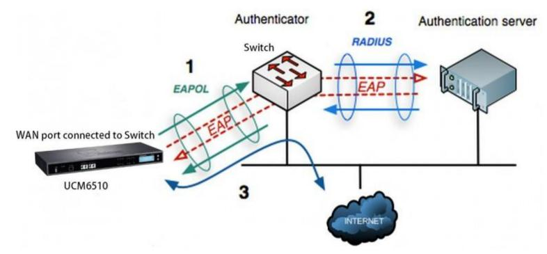
Figure 15: UCM6510 using 802.1X as Client
