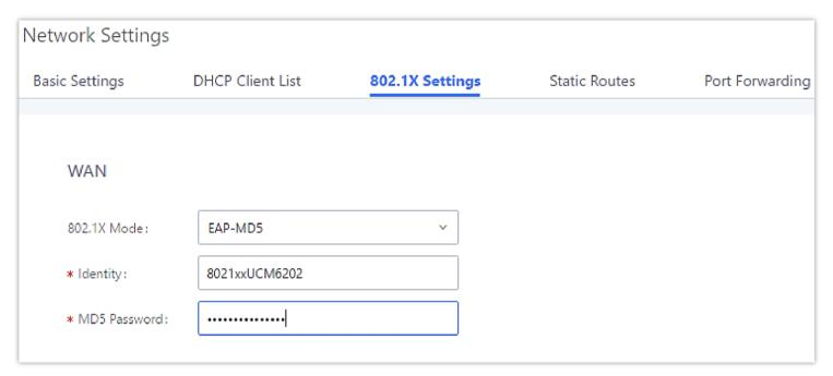
Figure 16: UCM6510 using 802.1X EAP-MD5
