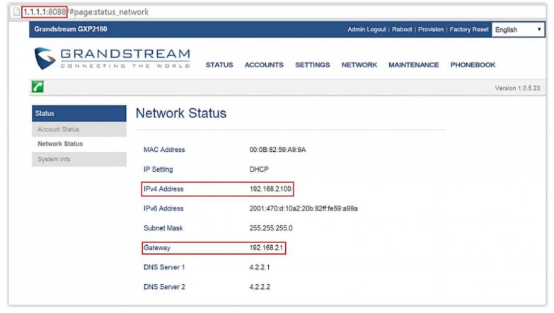
Figure 21: GXP2160 Web Access Using UCM6510 Port Forwarding
