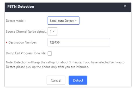
Figure 101: UCM6510 PSTN Detection: Semi-Auto Detect
