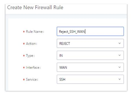
Figure 26: Create New Firewall Rule
