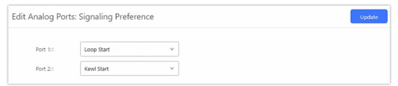
Figure 102: FXS Ports Signaling Preference
