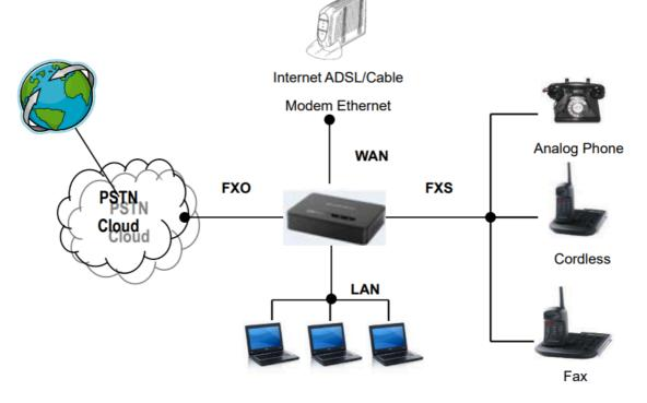
Figure 3: Connecting the HT813
