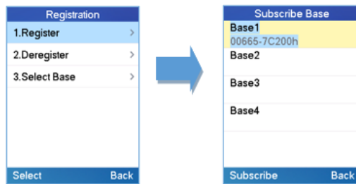
Figure 12: Multiple Base Stations Registration
