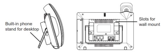
Figure 2: Built in Stand and Mounting Slots on The GXV3370.
