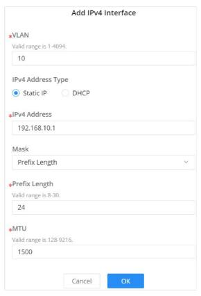
Add VLAN IP Interface - Static IP
