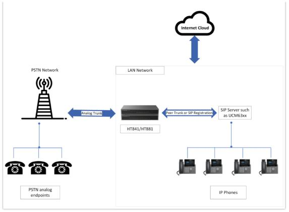
Functional Diagram of IP-PBX & HT841/HT881
