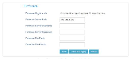
Figure 18: Upgrade Configuration via Web GUI
