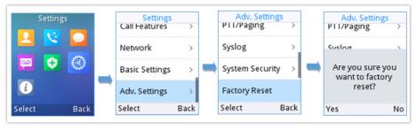
Figure 19: LCD - Confirm Factory Reset
