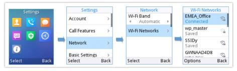
Figure 10: Connecting to Wi-Fi Network
