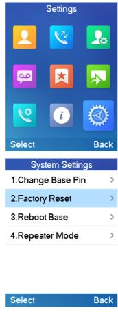
Figure 37: Resetting the Base Station
