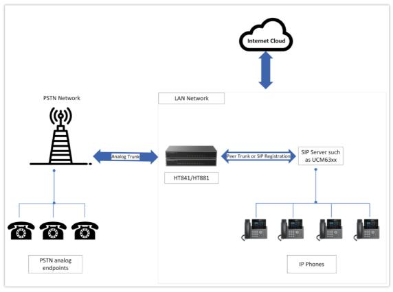
Functional Diagram of IP-PBX & HT841/HT881
