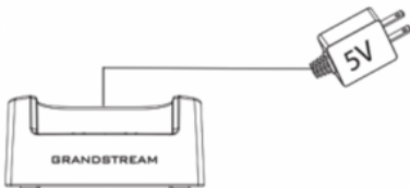
DP722 Charging Station
