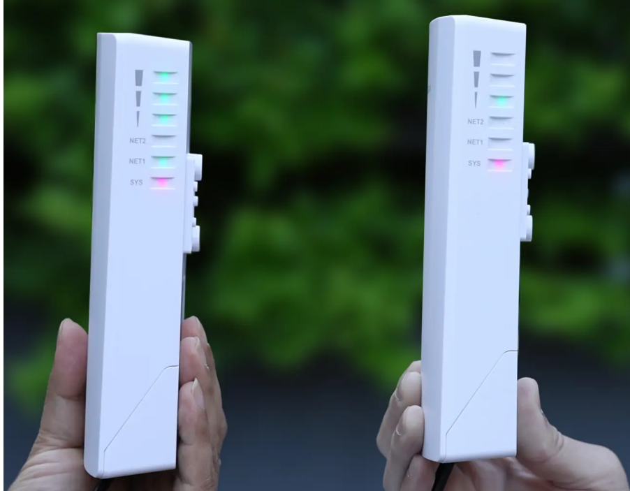
Step 3 Slave device right pairing in progress
