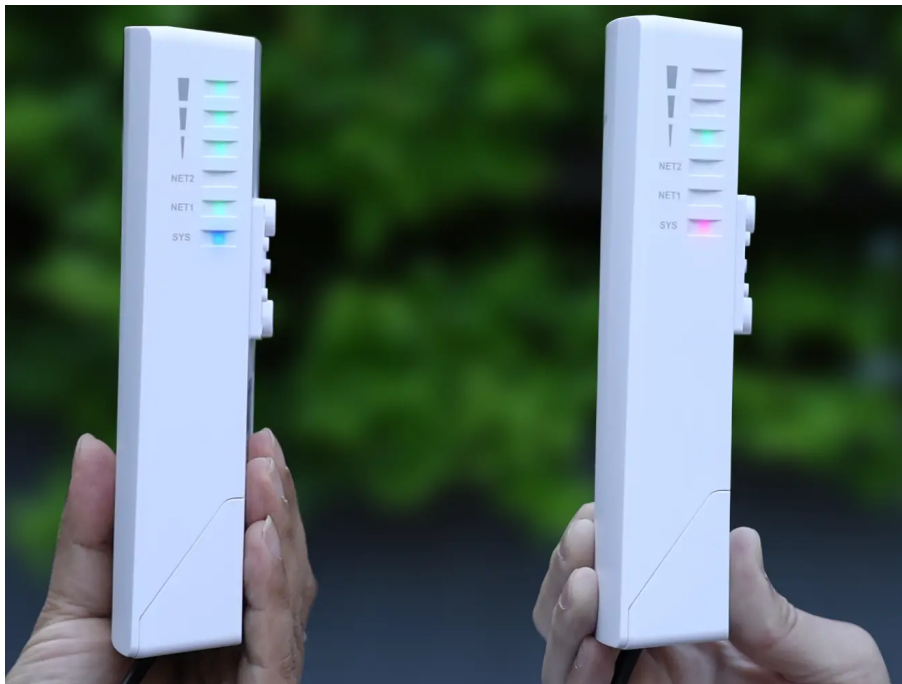
Step 2 Master device left after pressing the RSTPAIR button 3 times
