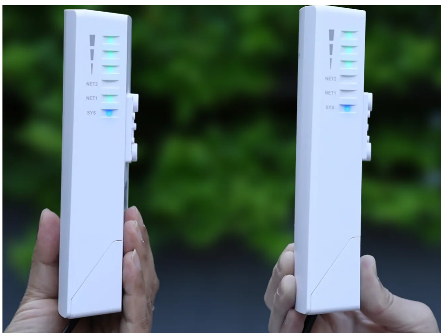
Step 3 Final status Master and Slave paired successfully SYS LEDs solid blue
